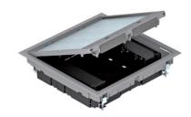
GES9 service outlet with a fixed construction height of 55 mm. With two fitted plug housings for vertical mounting of Modul 45 devices and four strain reliefs. Two installation frames are required to mount Modul 45 devices.
