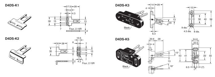
With Operation Key Inserted (Relationship between Insertion Radius and Insertion Hole) **Note:** Unless otherwise specified, a tolerance of ±0.4 mm applies to all dimensions.
