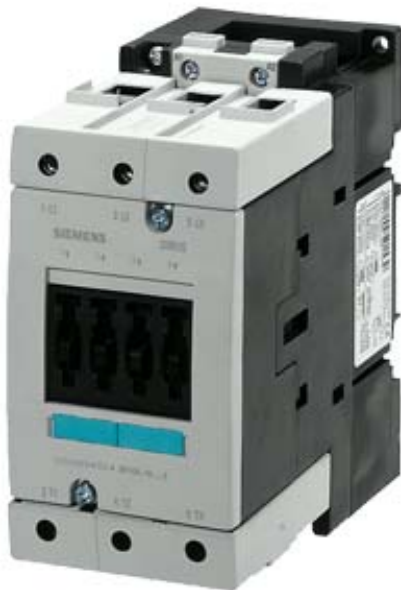
CONTACTOR, AC-3 30 KW/400 V, AC 220V 50/60HZ 3-POLE, SIZE S3, SCREW CONNECTION
