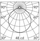
Luminous flux luminaire 124 lm
